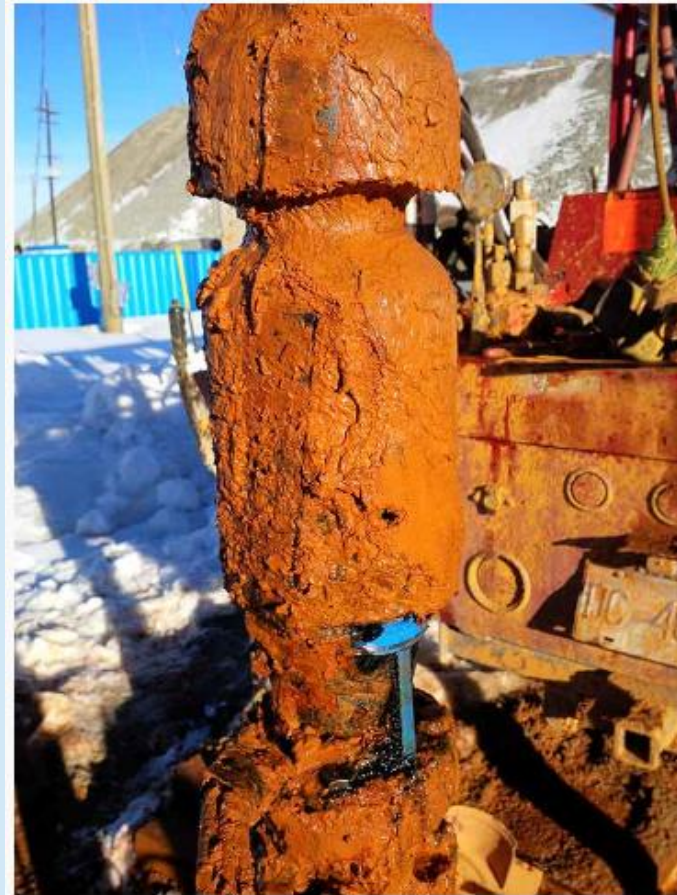
Image 1 of 2 Biofouling is caused when naturally occurring bacteria interact with the components of the well and form a slimy deposit often referred to as iron bacteria. Photo courtesy of Ingram Well and Pump Service
